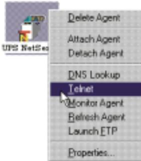
1) Select the device required by right clicking on the UPS icon on the PeripheralVision® network map. This will open the menu displayed here.
