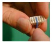
1) Place the wire into the required slot of the IDC connector
