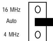
The red jumper will be over the **Auto** pin only, enabling the monitor to select 16MHz or 4MHz as required. To set one speed only, remove the jumper and replace it over the **Auto** pin *and* the pin of the speed you wish to set, as shown in the diagrams below.
